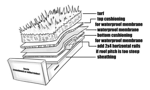
On top of your roof sheathing you will lay your impermeable layer. This is the most important part of your living roof because it keeps water out of your building. There are many permeable membranes available, but one of the most reliable and highly recommended membranes to use is an EPDM. They are very durable and resistant to piercing. They will also last for at least 50 years underneath soil.
