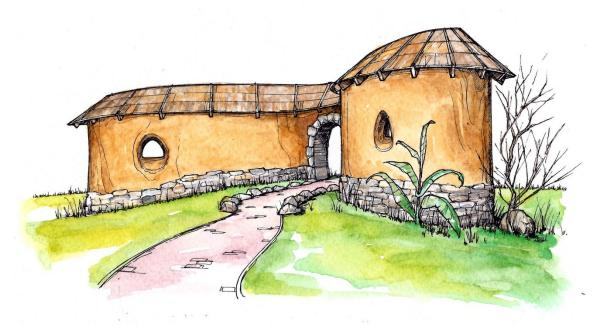
A garden wall is a good project to begin cobbing with too. You will learn how to dig and construct a rubble trench foundation, set a stem wall foundation, mix and apply cob, and
