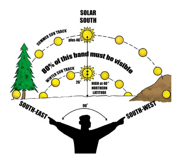
The orientation of the building and the placement of windows are important design elements that must be taken into consideration when using passive solar. The intelligent placement of windows is important so that you can get enough sunlight to penetrate inside the building. The sunlight that you want to capture will mainly come from the south, southeast, and sometimes from the east.
