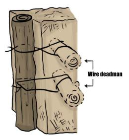
The best way to install doors is to set the door frame in place before you build the cob walls. Connect the bottom of the door frame to the foundation, cross brace and anchor it, then build the cob walls up around the frame burying your anchors as you go.
