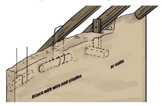
Bury a deadman about two feet below the end of each rafter and ridge beam. Use a thick piece of wood about 18" long such as a thick branch or piece of wood. Use a strong galvanized wire, wrap it around the deadman twice, and staple it on securely. Electric fencing wire or any other heavy fencing wire is a good option.
